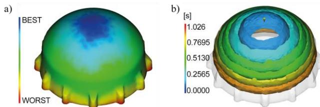
Fig. 1. Gate location (a) and expected flow direction during the filling process (b)
