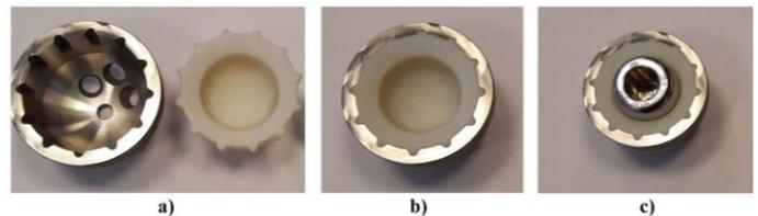
Fig. 11. The injection moulded UHMWPE liner in the acetabular component
