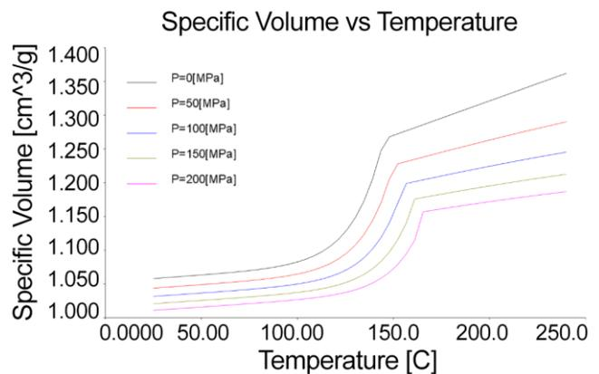
Fig. 3. Pressure-volume-temperature curve of UHMWPE
