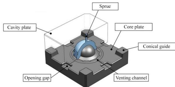
Fig. 7. Injection mould design
