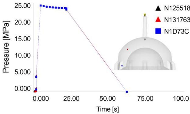
Fig. 4. Mould cavity pressure as a function of time at different distances from the gate
