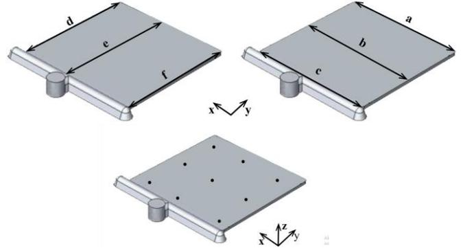
Fig. 6. Average linear shrinkage from distance and thickness measurements
