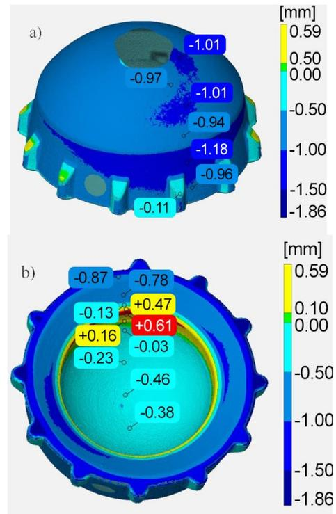
Fig. 10. Comparison of the original CAD models and the injection moulded parts: (a) outer and (b) inner geometry
