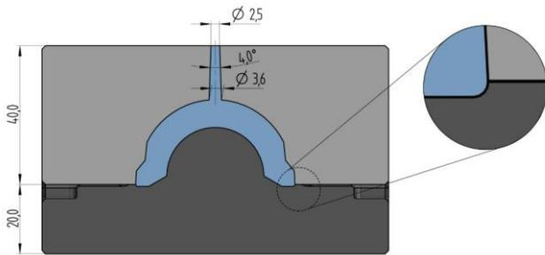
Fig. 8. Section view of the mould with main dimensions
