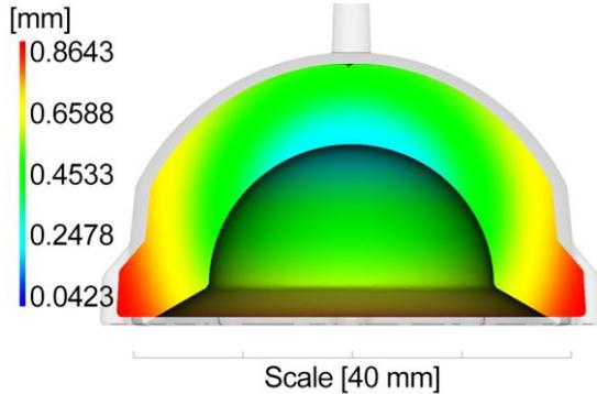
Fig. 5. Expected size change of the liner after injection moulding
