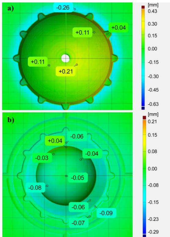
Fig. 9. Comparison of the CAD models and the 3D scanned mould halves
