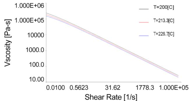
Fig. 2. Viscosity curve of UHMWPE
